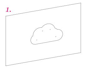
Use blu tack or tape to place template on wall ensure template is straight using a spirit level
