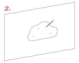
Mark out screw holes on the wall
