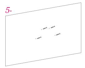
Place screws into rawl plugs leaving 1cm of screw out
